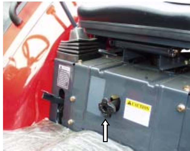
FIG.2-23 Slow return check valve
