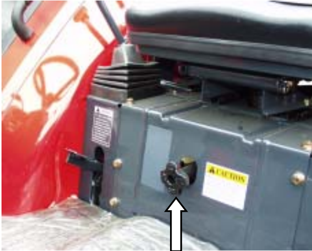
FIG.2-40 slow return check valve knob
