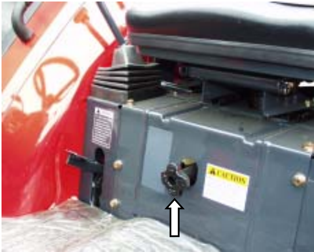
FIG.2-31 Slow return check valve
