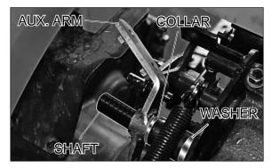
3.Install liner, conical spring and nuts (M16) to the shaft.
