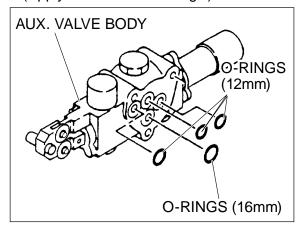
2.Installelbow to the Aux. valve body. Tighten the elbows to the following torque.43.4-50.6Lbf ft (59-69N-m)
