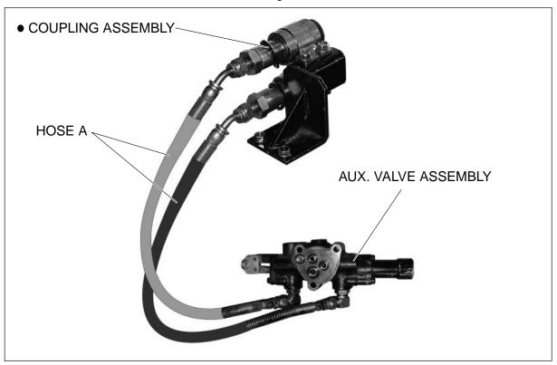
5.The hose A is connected as shown in the figure below.
