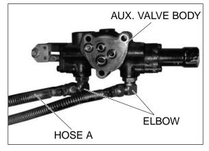
5.Set the cap, plate, O-ring with three bolts (M8x85mm:2pcs, M8x140mm:1pcs) and washers to the Aux. valve body.
