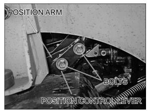
2.Install tube to the position control lever.
