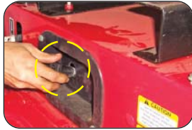
Removing of Control Levers Knob
