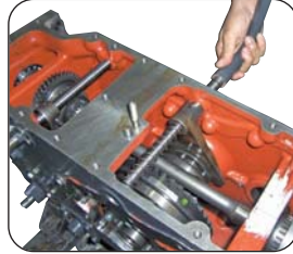
Assemble Diff. Lock Shaft
