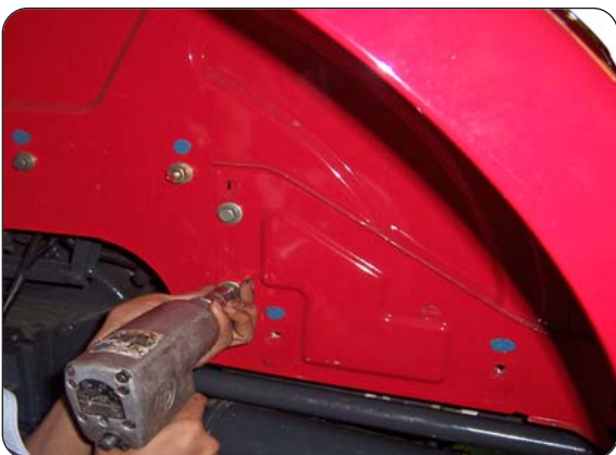
Removal of Fenders
