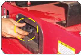
Removing of Control Levers Knob
