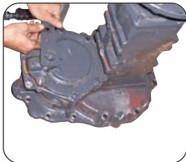
Removal of Cover Plate Brake
