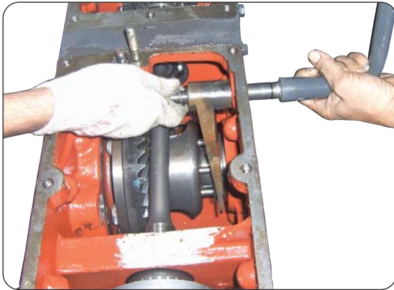
Special Tool Removal of Differential Lock Shaft Pin
