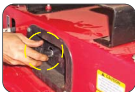
Removing of Control Levers Knob
