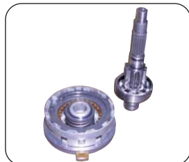
Removal of Input Shaft from Wet Clutch
