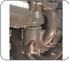
Swivel Housing Oil Drain Plug
