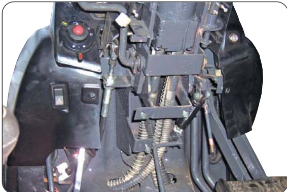
Steering Column Cover Removed
