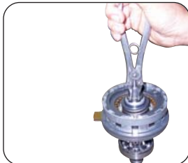
Removal of Input Shaft from Wet Clutch
