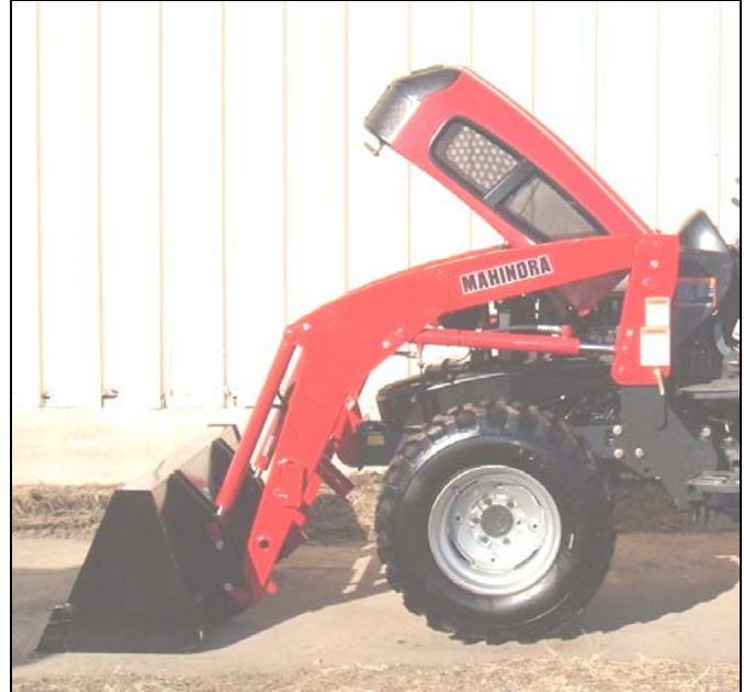
B. Position loader with bucket and/or attachment level with ground, then relieve all hydraulic pressure.
