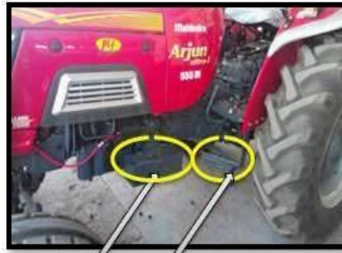
Tool box Stair
