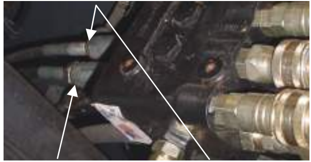
Install Dump and Rollback (Tilt) Cable to Lower Spool of Valve
